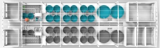
Fig. 1. Layout design for the Recirculating Aquaculture System complex at SAU
